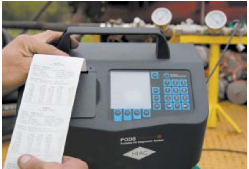
[ABOVE] On-line particle counters and real-time readouts tell operators when ISO cleaning specifications have been met without the downtime associated with conventional testing.
